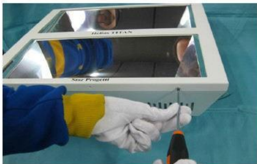
1. UNSCREW THE SCREWS HOLDING THE FRAME.
