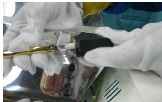
6. RECONNECT THE FASTONS ON THE NEW BULB AND APPLY THE SILICON SEALS TO THE BULB.
